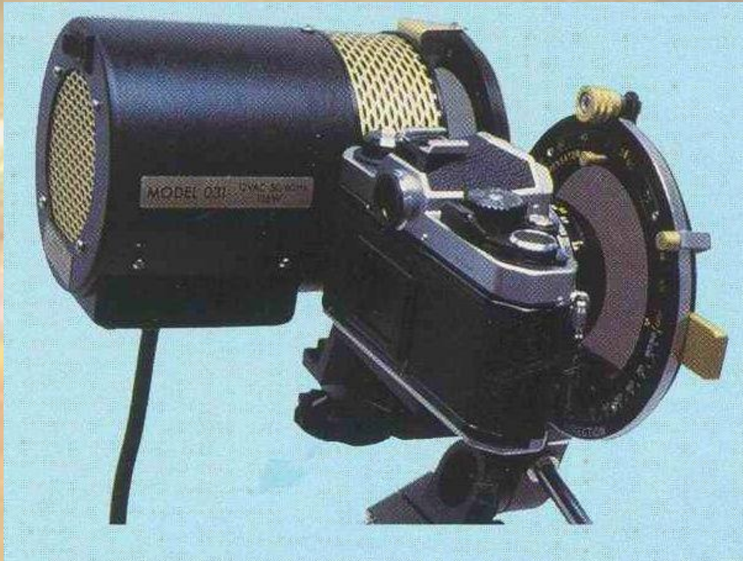
*Vishay, Series B 031, reflection polariscope
